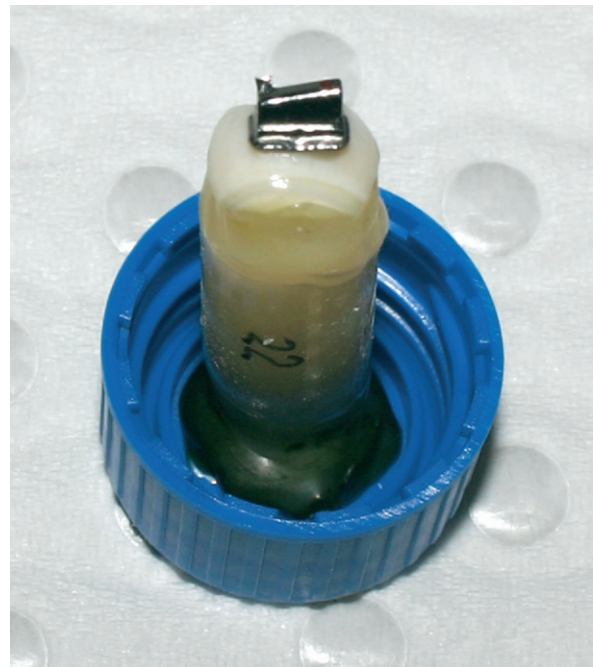
Fig 1. Prepared enamel specimen mounted on sticky wax stick and bonded with molar tube.
